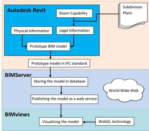
**Figure 10** The approach for preparing and visualizing the prototype BIM model
