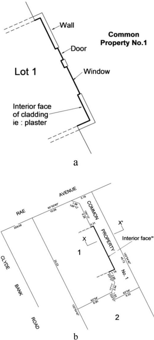
**Figure 4** Boundaries referencing physical structures: (a) Physical elements within building; and (b) Plan depiction (LandVictoria 2012)
