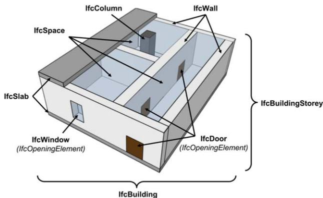
**Figure 8** Physical information in the IFC standard, adapted from (Nagel 2014)
