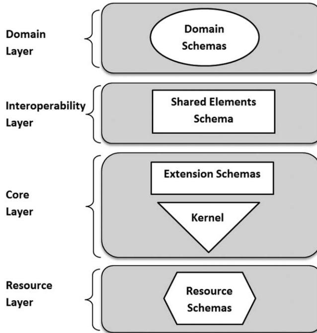
**Figure 5** Simplified conceptual data schema of the IFC standard, adapted from (ISO 2013)
