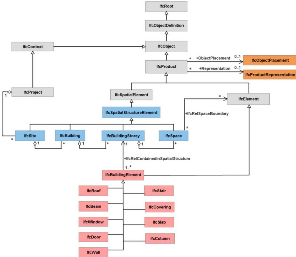
Figure 7 Physical data entities in IFC data model
