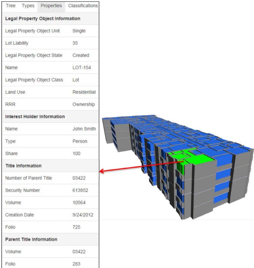
Figure 11 Managing the legal information in the developed prototype BIM model
