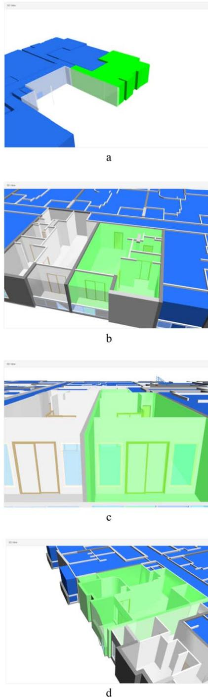
**Figure 12** Significance of physical information in communicating different ownership boundaries: The type of boundary cannot be determined by only legal spaces (a); interior wall boundary (b); middle wall boundary (c); and exterior wall boundary (d)
